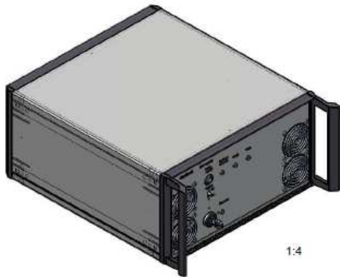
Controller (height = 184; width = 343; length = 375 core dimensions in mm )
