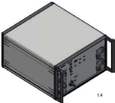
Controller (height = 184, width = 343; length = 375 core dimensions in mm )
